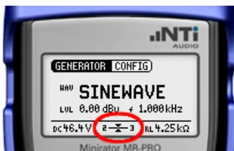
Plug the MR-PRO into the down-line section of the path (towards the mixer). Select 1kHz SINEWAVE and check that the down-line signal is balanced, because a missing screen on the cable or an unbalanced line can often cause the hum.
