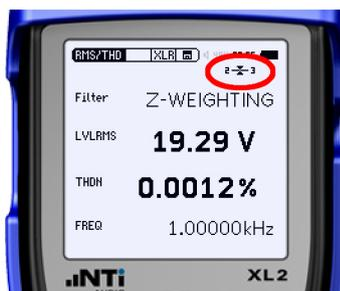
At the same point in the signal path, plug the XL2 into the up-line section of the path (from the mic or instrument). Select RMS/THD, create a sound at the source (ask the guitarist to play or gently tap the microphone) and check that the up-line signal is balanced. Press the speaker button on the XL2 and listen for the hum through the XL2 internal speaker.
