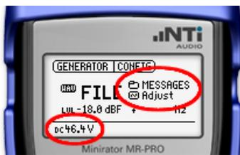
Confirm that the line is providing phantom power to the microphone if appropriate. (The DC value should be  $48V \pm 4V$ )
