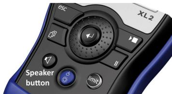
Interrupt the signal path at various points, plug the XL2 into the up-line section of the path (from the MR-PRO). Select SLMeter. Press the speaker button on the XL2 and listen for the signal from the MR-PRO through the XL2 internal speaker. To adjust the volume, hold the speaker button and turn the wheel.
