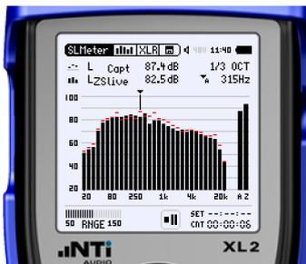
Position the XL2 microphone at the nearest audience position in front of the right (or center) speakers. Release the pause to measure LZSlive. Adjust the frequency response until the spectrum is similar to the reference spectrum of the left PA (the left PA Capture is shown here in red).
